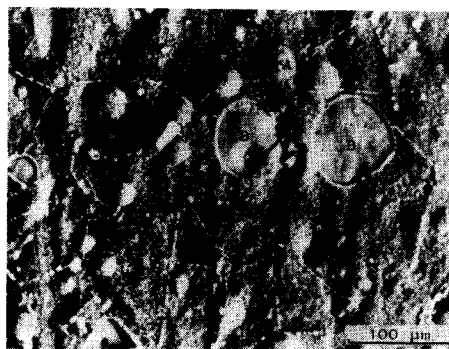
Fig.2. The backscattered electron image of silver grains obtained from the scanning electron-microscope autoradiograph of tritium on Cu-Ni(1:1) alloy.
