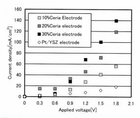
Fig.3 Current density of electrodes against applied voltage
