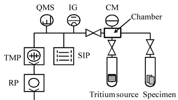
Fig. 2. Schematic view of tritium exposure apparatus.
