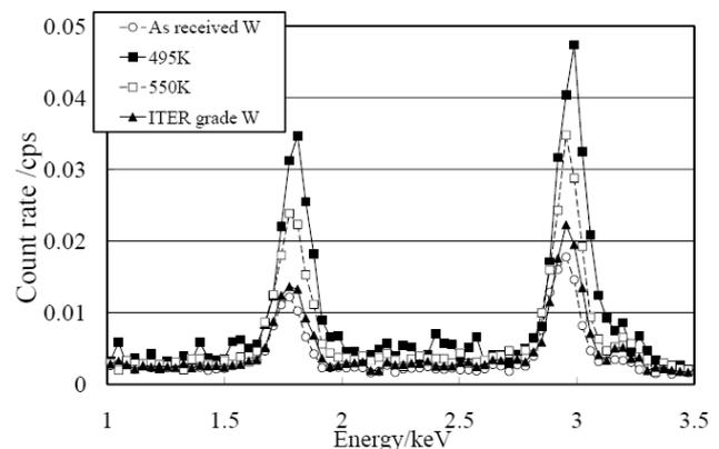
Fig. 4. BIXS measurement results of each specimen
