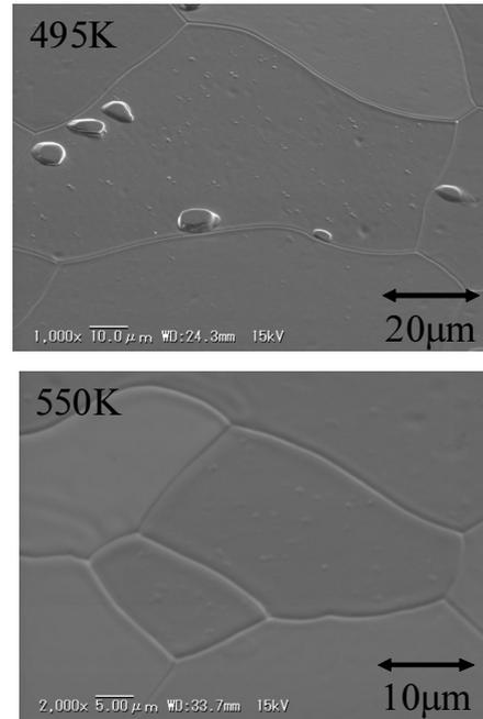
Fig. 3. Surface observations result after D plasma exposure
