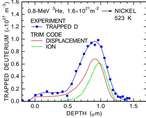
Fig.3 The depth profile of trapped deuterium obtained from the data shown in Fig.2.<sup>5</sup> Distribution of bombarding ions and atomic displacements are also shown.
