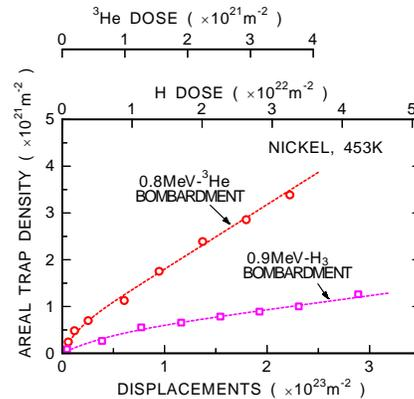
Fig.7 Evolution of the trap density with atomic displacement in nickel.<sup>9</sup>
