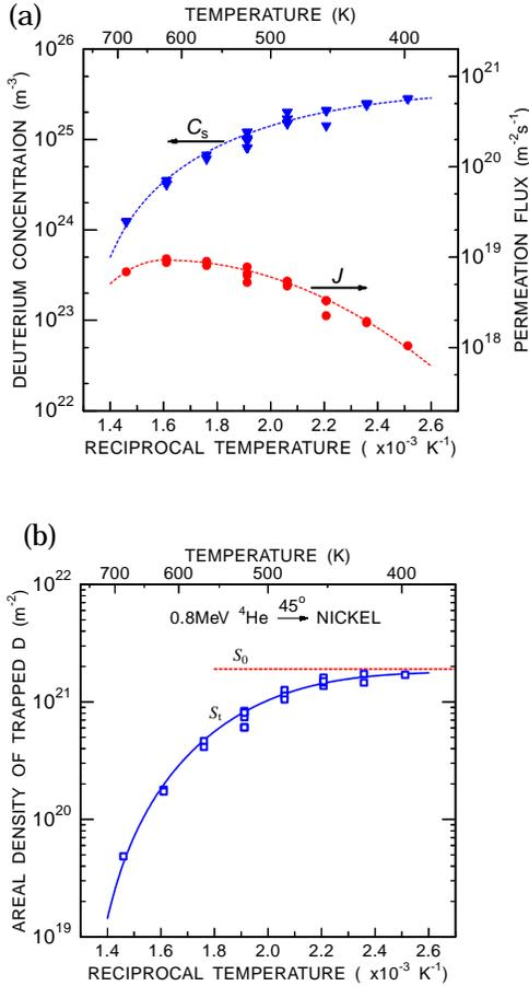
Fig.5 Temperature dependence of (a) the concentration of dissolved deuterium and (b) the areal density of trapped deuterium in nickel bombarded with  $^4He$ .<sup>3</sup>
