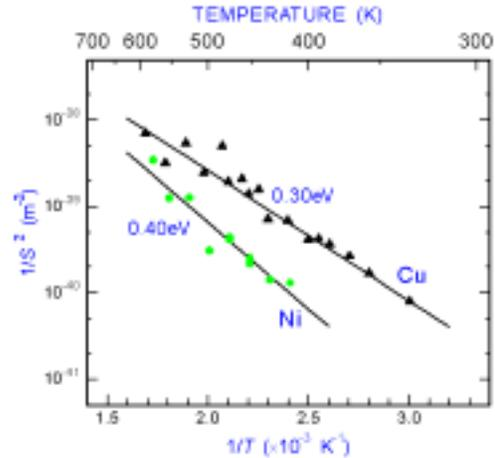
Fig.10 Temperature dependence of  $1/S^2$  on nickel and copper membranes.<sup>11</sup>
