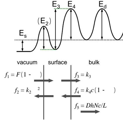
Fig.9 Schematic showings of potential energy diagram and rate processes of hydrogen near metal surface.
