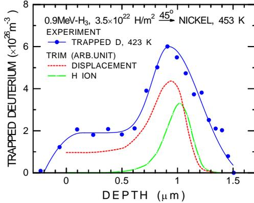
Fig.4 The depth profile of trapped deuterium in nickel bombarded with hydrogen ions.<sup>7</sup> Distribution of bombarding ions and atomic displacements are also shown.
