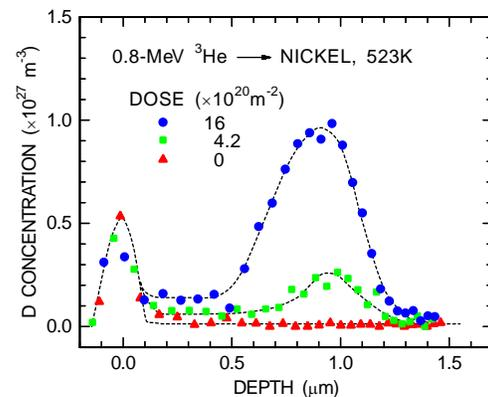
Fig.2 Depth profiles of deuterium in nickel before and after 0.8MeV-<sup>3</sup>He bombardment.<sup>5</sup>
