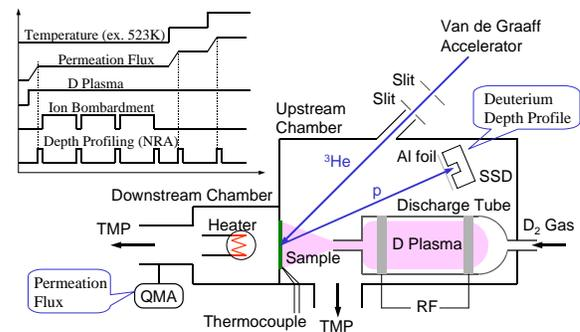
Fig.1 Schematic illustration for the experimental setup and its typical procedure
