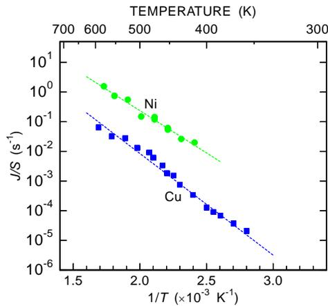
Fig.11 Temperature dependence of  $J/S$  in nickel and copper membranes.<sup>11</sup>
