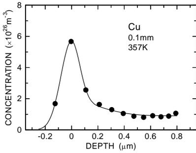
Fig.8 A typical depth profile of deuterium in a copper membrane exposed to deuterium plasma.<sup>10</sup>
