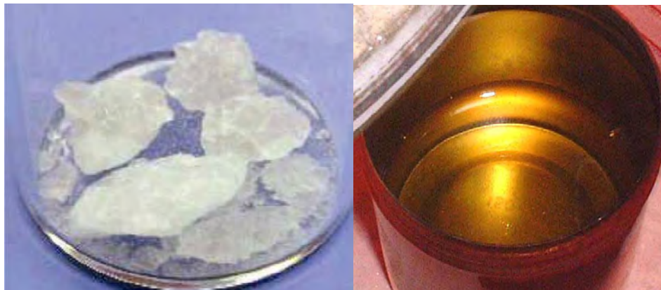
Fig. 1 Photos of solid Flibe at room temperature and transparent molten salt when its melts
