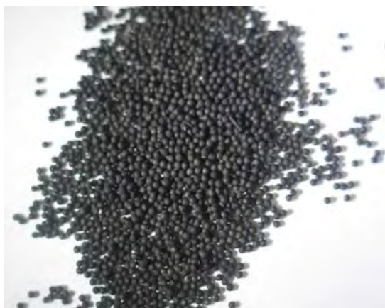
Fig.3 Appearance of 1.0 wt% Pt/ \text{Li}_4\text{SiO}_4 pebble
