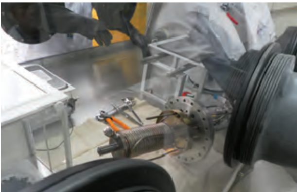
Fig.1 Hydride bed in the glovebox [5].
