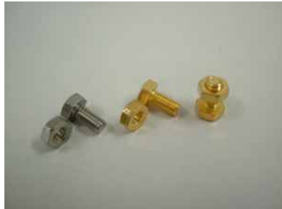
Fig. 2. Showing the bolts and nuts before (left) and after (center) Au coating with a good fitting (right). Sputtering conditions; 100W, 1 h.
