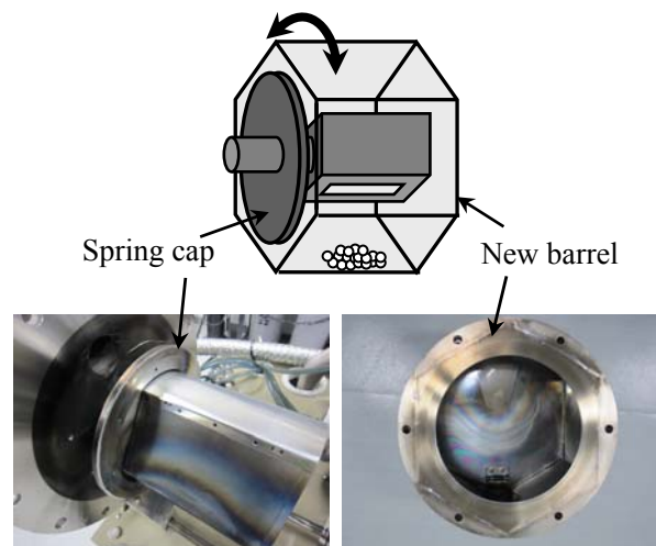
Figure 5 Schematic figure of the redesigned polygonal barrel-sputtering system and photographs of its components.
