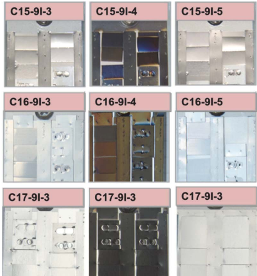
Fig. 2 Pictures of coupons placed near 9I ports in the LHD campaigns C15, C16 and C17.
