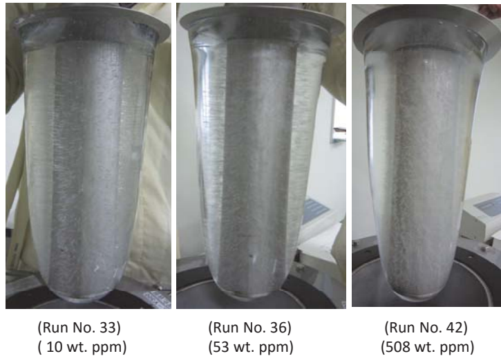
Fig. 9 Photos of ice formed for various concentration of NaCl.
