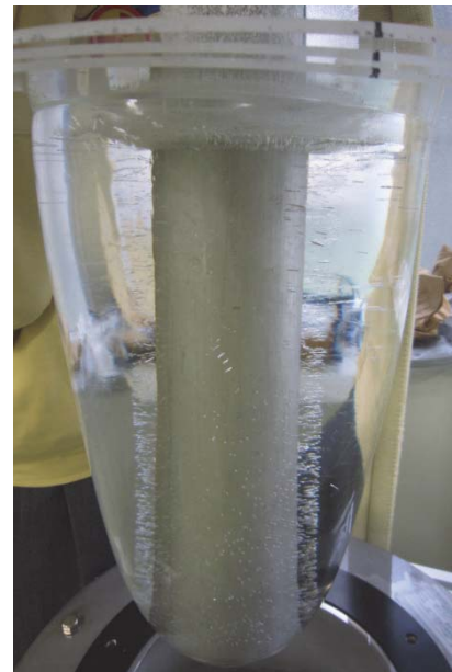
Fig. 3 Example of the ice produced in the freezing vessel (Run No. 10).
