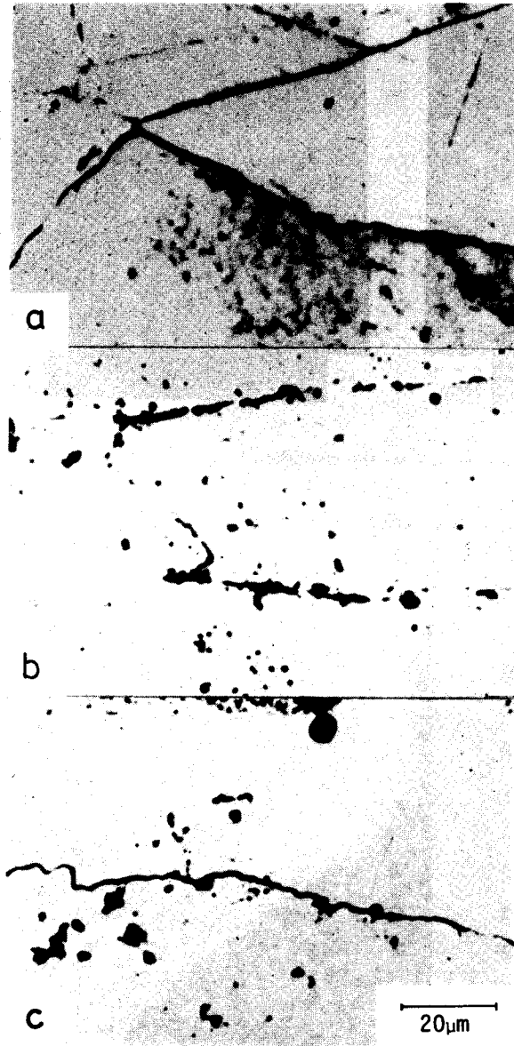
Fig. 5 Microphotograph showing; (a) the microstructure after etching, (b) and (c) autoradiographs of the cold rolled specimen.
