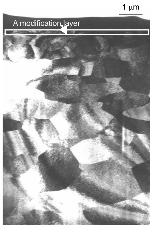
Fig. 5 XTEM image of W sample after 7 eV deuterium plasma exposure.
