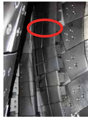
Fig.1 Photo of inner divertor region of Large Helical Device (LHD) in National Institute of Fusion Science (NIFS). The circled tiles are those analyzed in this study; the tile in right side is 9RD16-1, and one in left side is 9RD16-2.
